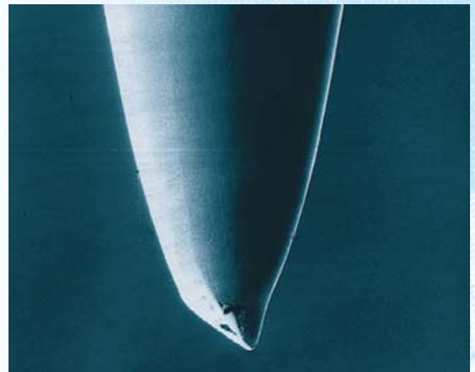
Damaged needle point Source: Groz-Beckert KG
